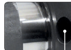
LIGHTENING HOLES IN ALL ROD JOURNALS
