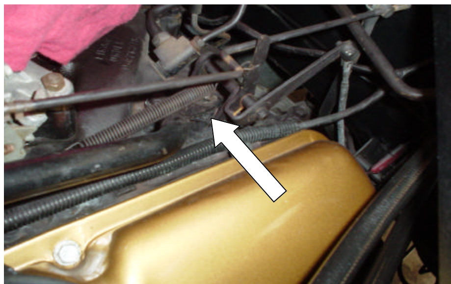
Figure 25. Stabilizer bar installation
