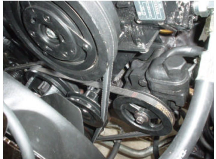
Figure 17. Eaton pump mounting bracket.
