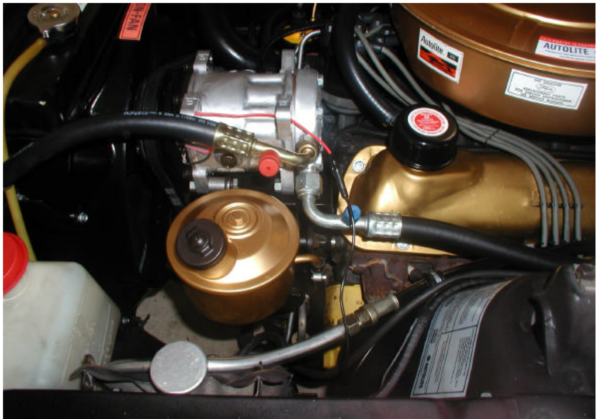
Figure 82 Aluminum liquid line routing
