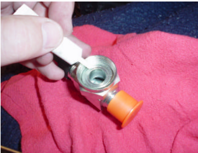
Figure 20 Apply 3 in 1 oil to the service valve threads.
