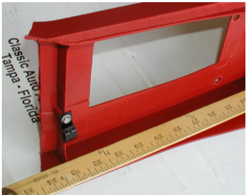
Figure 96 Measuring new console length
