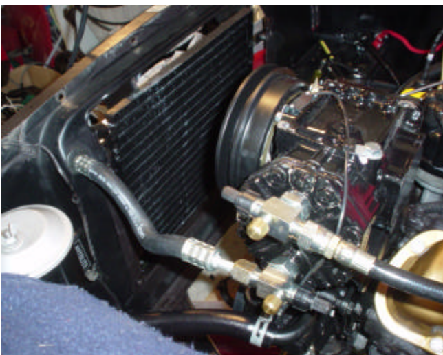
Figure 21 The completed installation should look as shown. Not the bend in the compressor to dryer hose. This is correct.
