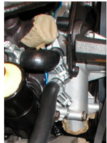
Fig. 15 Covered water pump openings
