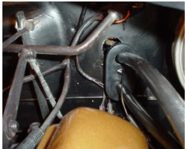
Figure 22 Route hoses through firewall.
