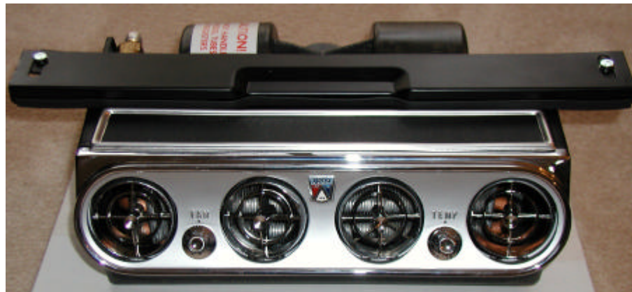
Fig. 60 Evaporator front view showing mounting ears
