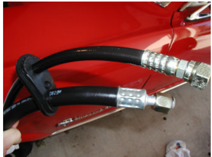
Fig. 55 Evaporator lines in firewall grommet
