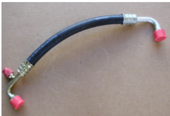
37. Compressor to Condensor Line
