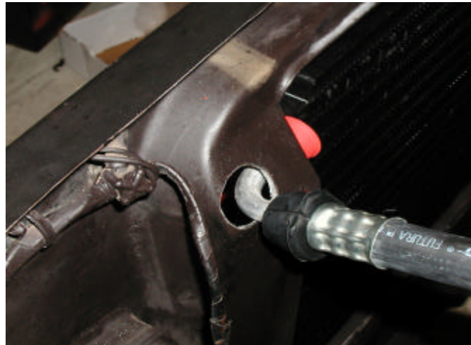
Fig. 34 Hole drilled in upper radiator support
