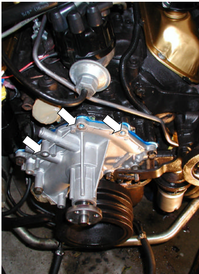
Fig. 25 Water pump mounting bolts needing removal.
