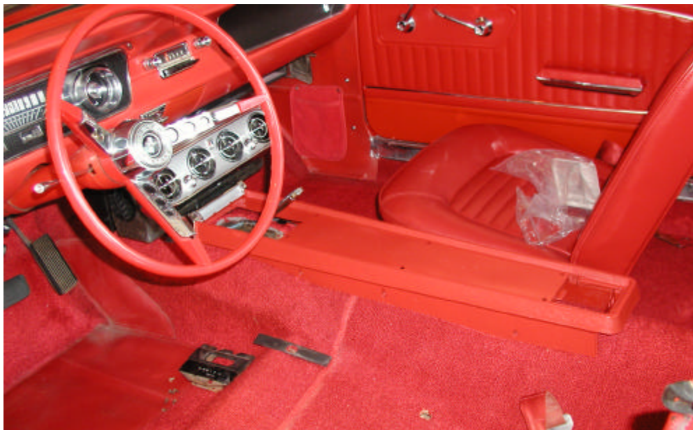
Figure 100 Painting cut console installed for test fit.
