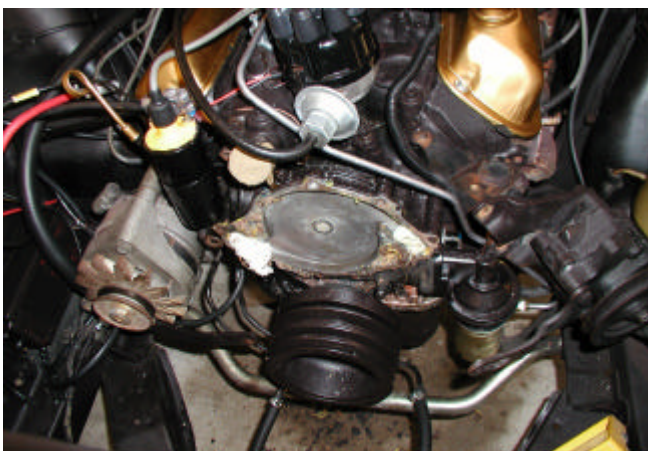
Fig. 10 Aluminum water pump removed.
