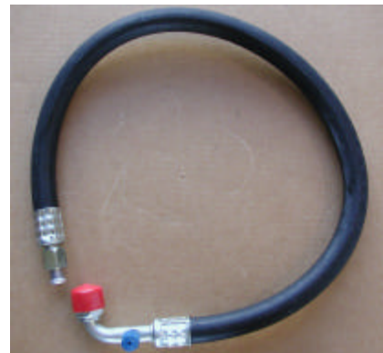
36. Low Pressure Line (Evaporator to Compressor)
