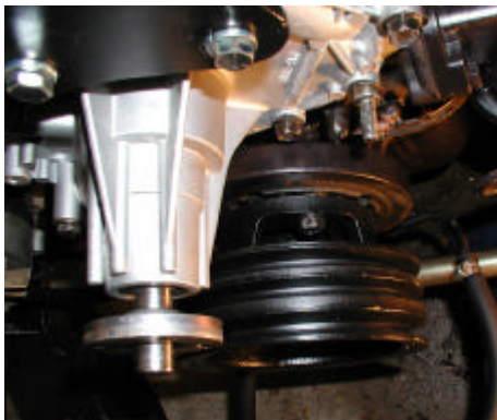
Fig. 41 New crankshaft pulley installed
