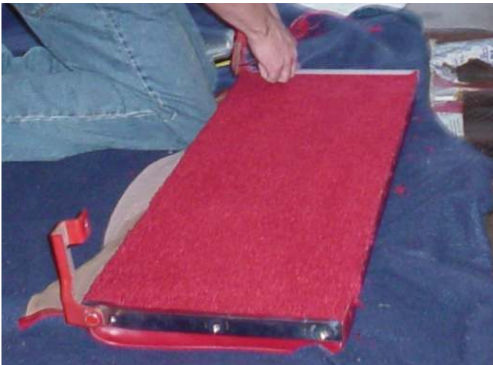
Figure 92 Replace all chrome after the carpet in is place and trimmed.
